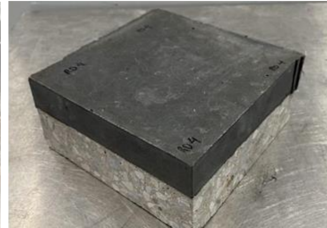
Characterization of the concrete to concrete interface
