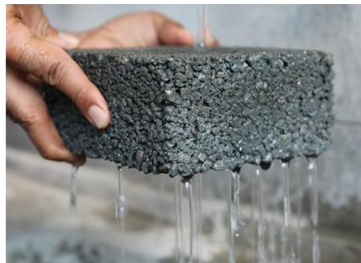
Water permeable pavers
